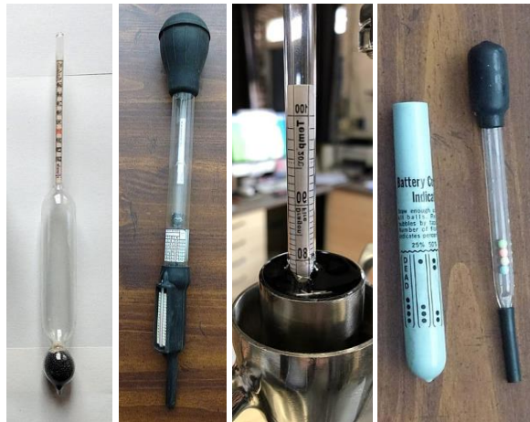
Figure 1: Examples of hydrometers: from left to right: lactometer, antifreeze meter, alcohol meter, battery tester (filled with mercury or other high-density materials: Food museums of the province of Parma 2019, Butch 2015b, Michel 2017, Butch 2015a)
