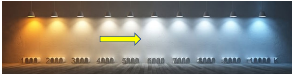
Figure 4. Movement along the curve in (a) results in changes in the CCT of white light in (b)
