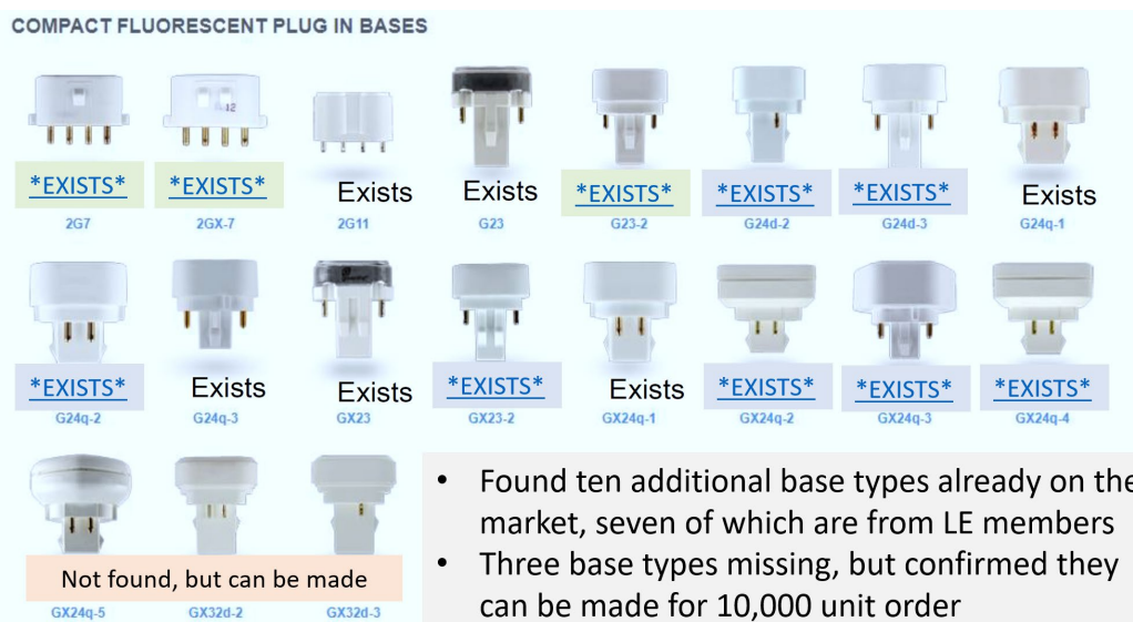
Figure 7. Illustration of the variety of CFLni base types and compatible LED Retrofit Lamps
