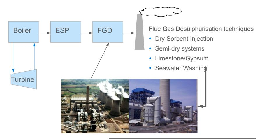
Mercury Impact: Improved collection of particulate and, especially, oxidised mercury – key part of any integrated environmental control strategy
