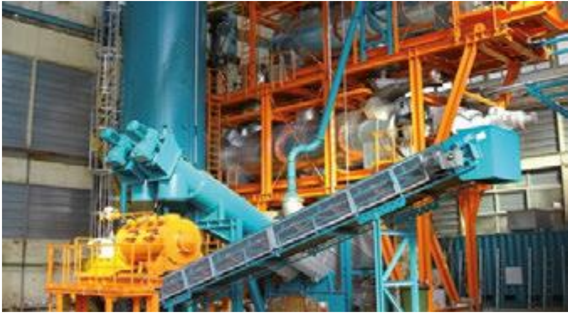
Indirectly heated vacuum distillation unit. Source: econ industries GmbH cited in UNEP/ISWA 2015
